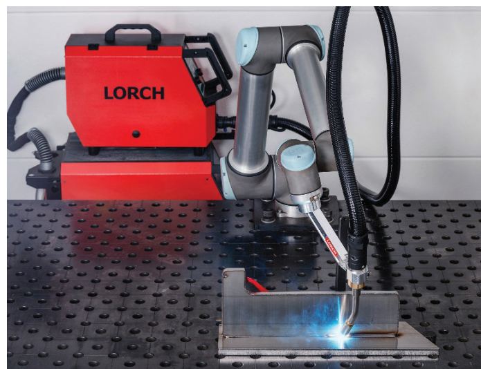
Fig. 3: Advantage automation: Once programmed, the Cobot will weld every seam with impeccable quality - even when used for a high volume of workpieces.
