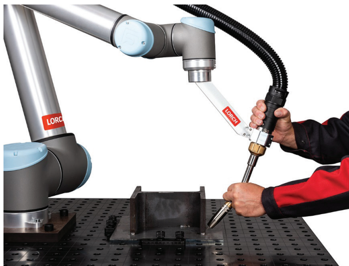
Fig. 2: Programming as easy as can be: Using the "Free Drive" function, the worker moves the operating arm to the positions where the welding process is supposed to start and end.
