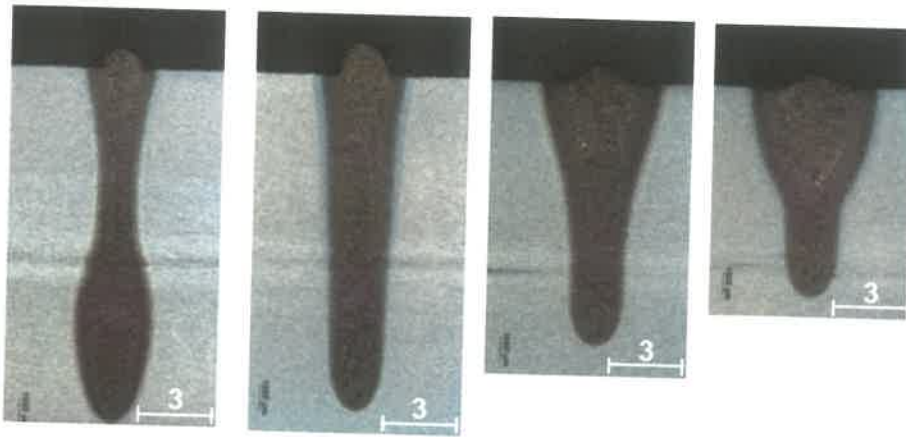
Figure 2 – Different weld geometries obtained at 10 mbar (a), 100 mbar (b), 500 mbar (c) and 1000 mbar (d) using unaltered laser parameter ( P = 5000 \text{ W} )
