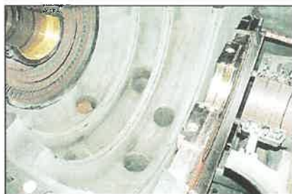
A high pressure steam turbine casing surfaces after reconditioning and coating. The technology is patented by Telatek.
