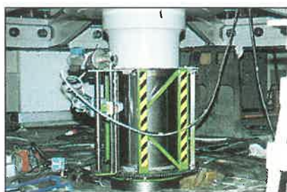
Mobile grinding and lapping equipment for bearing surfaces of electrical motors, steam and gas turbine rotors, generators, etc. The equipment is patented by Telatek.
